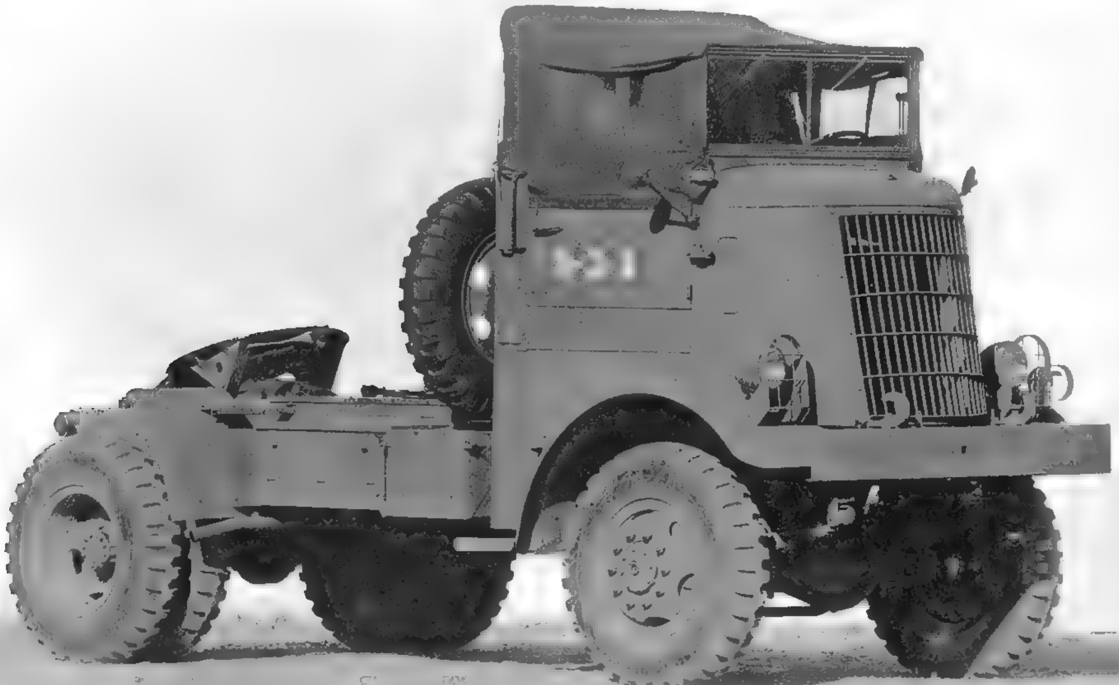
Canvas tarpaulins were provided with the open-cab 94x43B and C Federal trucks for weather protection, and a tool box was mounted on the right frame rail just behind the battery compartment. (U.S. Army photo)
